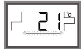
5. Room temp. setpoint (1)
